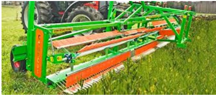
Figure 8: CombCut weed cutter
